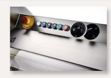
Push - button control The semi - automatic keyboard control is self - explanatory. It is very easy to operate. Simply press the button twice and turn the feed adjustment wheel once to start the machine.
